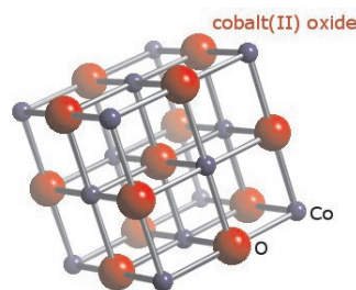
Fig. 12.4: Rock-salt (NaCl)-type structure of CoO.
