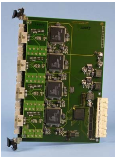
Fig. 1: TDC-board with 8 F1-chips. 64 channels in common stop mode, resolution 120 ps.
