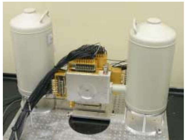
Fig. 2: The Compact Si+Ge Compton Camera at LLNL consisting of the double-sided strip Si(Li) detector (shown in Fig. 1) and a double-sided strip HPGe detector.
