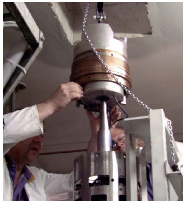
Fig. 5: Dismantling of the magnetic solenoidal lens close to the magnetic center of the injector cyclotron. The lower part of the magnetic center with the last focusing solenoid "LM" of the source beam line was lifted through the floor of the cyclotron hall.
