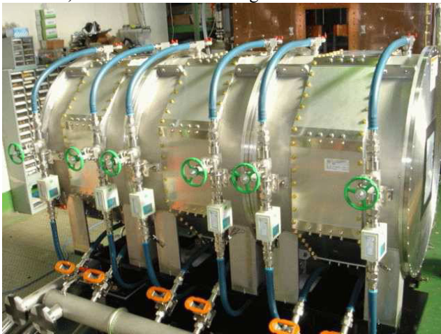
Fig.6 the optimized cavity structure for direct cooling
