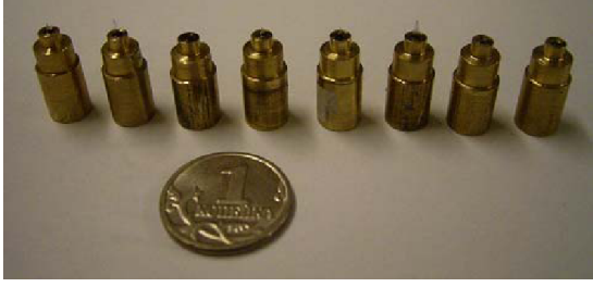
Fig. 57: Nozzles from quartz glass and brass for droplet production.
