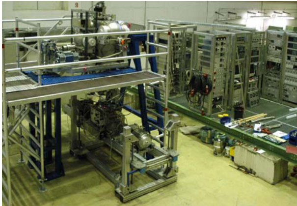
Fig. 56: The experimental setup in the “LKW-Schleuse” of the COSY hall: The ABS (vertical) in its horizontal support bridge, the LSP (horizontal) in the lower support system, and the ISTC chamber underneath the ABS. On the right-hand side the movable platform (green) with the supply units for ABS and LSP is shown.
