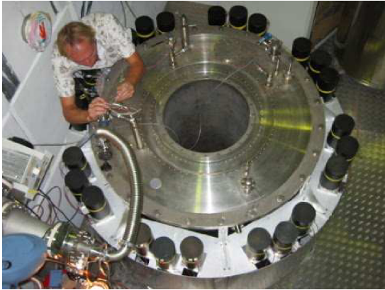
Fig. 26: ATRAP-II magnet and C. Storry during assembly.
