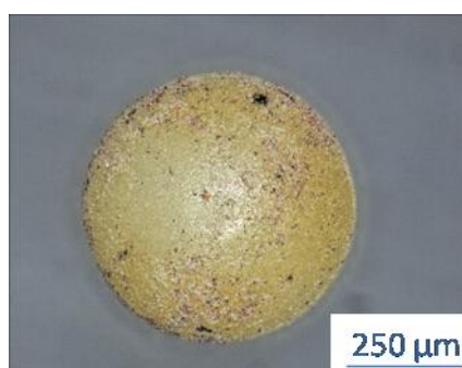
Figure1: (\text{Ce,Fe})\text{O}_x coated \text{ZrO}_2 beadlets.
