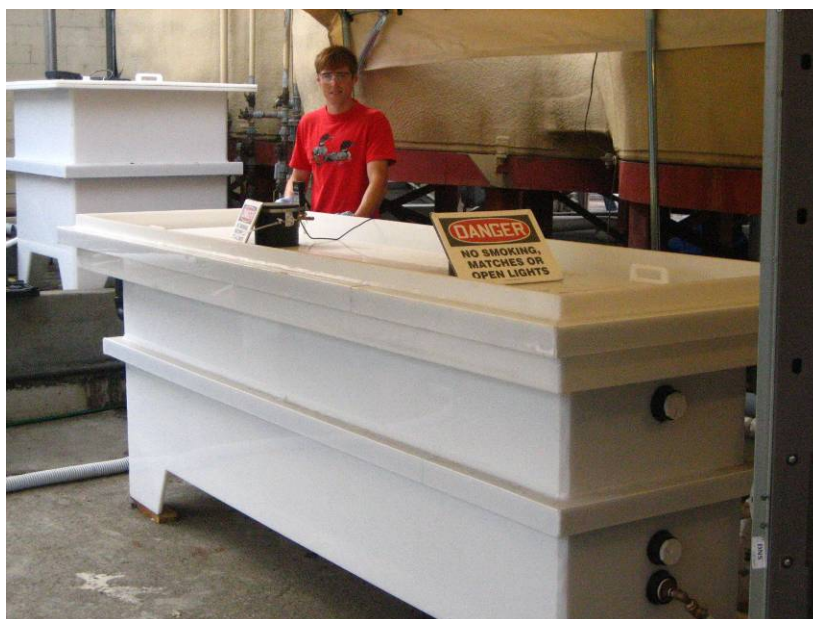
Figure 2: Photograph of a 1000-liter MEC being tested for hydrogen production using wastewater from a winery.
