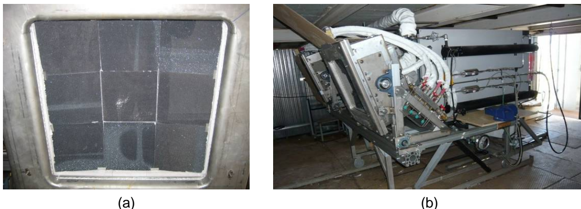
Figure 1: Pilot, 100 kW-scale HYDROSOL solar reactor: (a) front face of reactor's individual chamber consisting of nine SiC square-shaped blocks; (b) dual chamber reactor completely assembled and installed at the SSPS tower, ready for operation.
