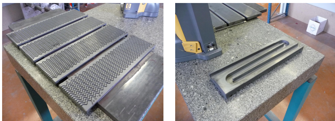
Figure 2: SiC channelled plates of the prototype: heat source plates (left) and a reaction plate with one large meandering channel (right).
