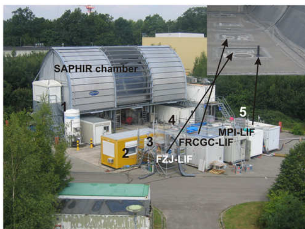
Fig. 1. Location of instruments during the HO x COMP campaign during ambient air sampling (labels in large photograph) and instrument inlets during SAPHIR experiments (arrows pointing to positions in the small photograph). Containers of MPI-LIF and FRCGC-LIF were moved underneath the chamber for SAPHIR experiments. HO 2 data in this work were delivered by FRCGC-LIF, MPI-LIF and FZJ-LIF. Numbers indicate positions of instrument inlets measuring: (1) NO x , O 3 , HCHO, VOC, H 2 O, CO (red sign: ambient measurements, green sign: SAPHIR measurements); (2) temperature, relative humidity, HONO; (3) ultrasonic anemometer; (4) filter-radiometer; (5) O 3 .
