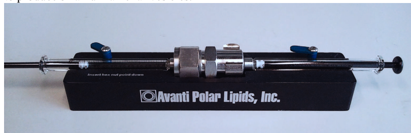
Figure 3.2: Avanti mini extruder used for production of SUV
