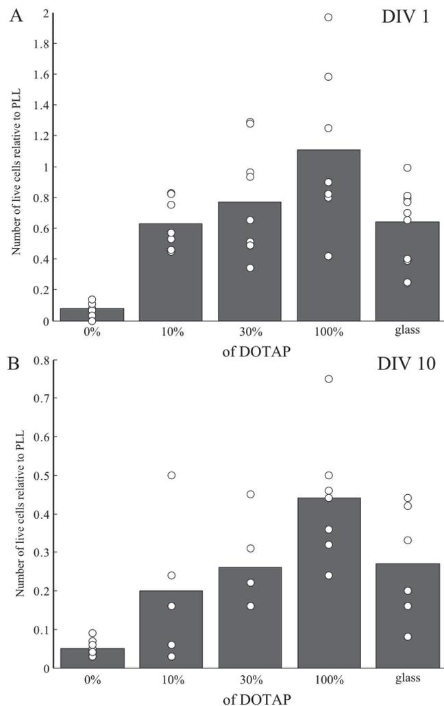
Figure 5.3: Number of live neurons growing on mixtures of POPC and DOTAP, as well as on uncoated glass for DIV1 (A) and DIV10 (B). The number of cells is normalized to the number of cells on PLL. The bars represent the average for each concentration. The circles are single measurements.
