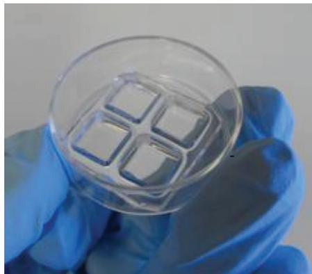
Figure 3.3: PDMS wells on glass slides used for the supported lipid bilayer (SLB) preparation.
