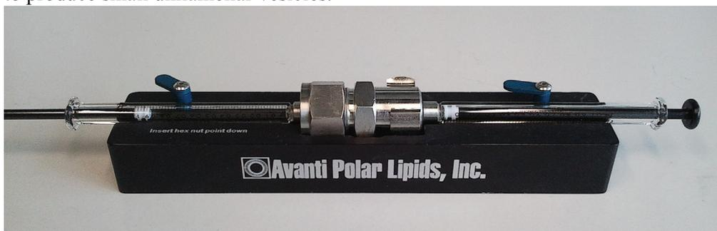
Figure 3.2: Avanti mini extruder used for production of SUV
