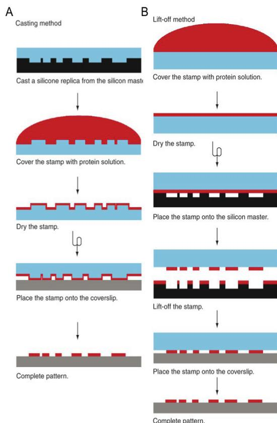
Figure 3.20: Two methods of microcontact printing [182]. (A) The casting method. A stamp is made by casting a silicone replica and then covered by ink. After drying the ink, the stamp is placed onto the substrate. (B) The lift-off method. Ink is dried on the surface of a polymer plate. Then the plate is placed on the silicon replica and after lift-off a pattern stays on the polymer. Then this pattern is transferred onto the substrate.
