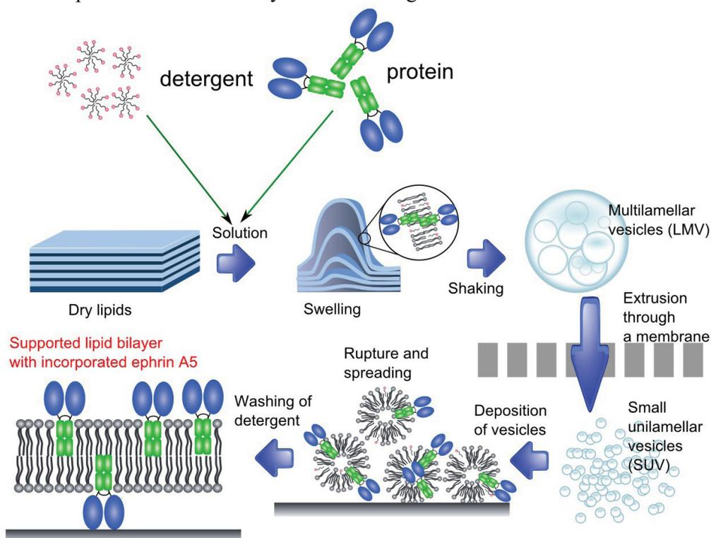
Figure 3.7: A schematic representation of preparation of the SLB with incorporated protein
