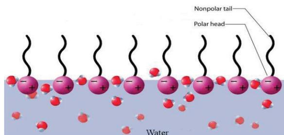
Figure 1.9: A monolayer of amphiphilic molecules arranged on the air-water interface [57].
