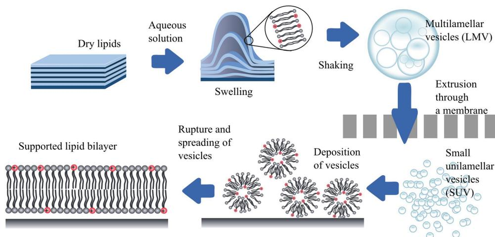
Figure 3.1: A schematic representation of the SLB preparation process including reconstitution of dry lipids in aqueous solution, formation of LMV, production of SUV by extrusion, vesicle deposition on the surface, their fusion and the SLB formation. Lipids of different types can be used. Positively charged lipids are marked by red colour. Zwitterionic lipids are grey.
