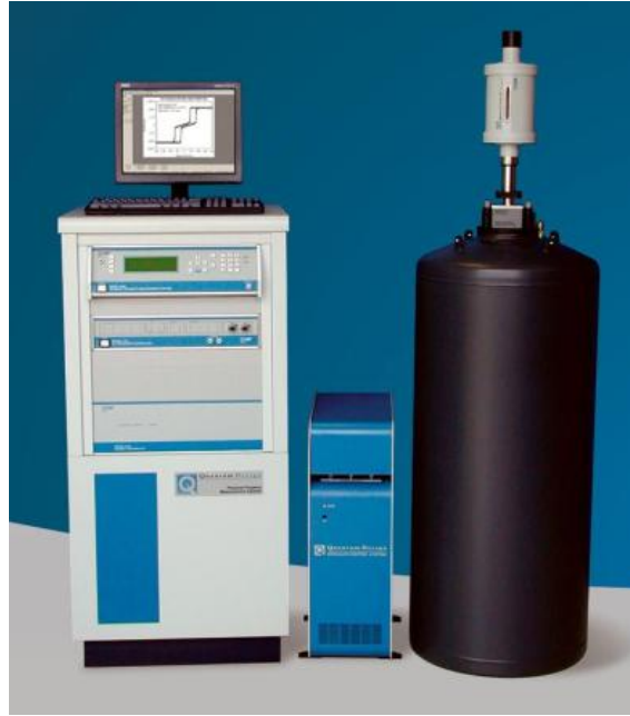
Figure 21: PPMS magnetometer with VSM option from Quantum Design [26].
