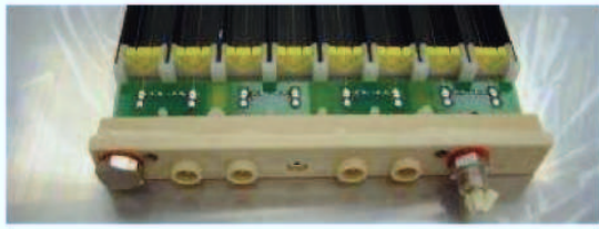
Figure 36: LST: Picture of a tube endcap with HV and gas connectors.
