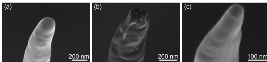
Figure IV.3.: SEM images of a flash cycle of a W-tip. (a) tip before flashing, (b) after short flash for 6 s at P = 1.6 VA and (c) after flashing for 18 s at P = 8.6 VA.
