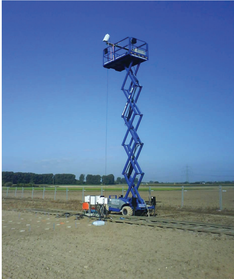
Figure 4.2: IR camera installed on an auto hoist 11 m above ground. The camera was used to measure the soil surface temperature of the experimental plot every 5 minutes during field experiment.
