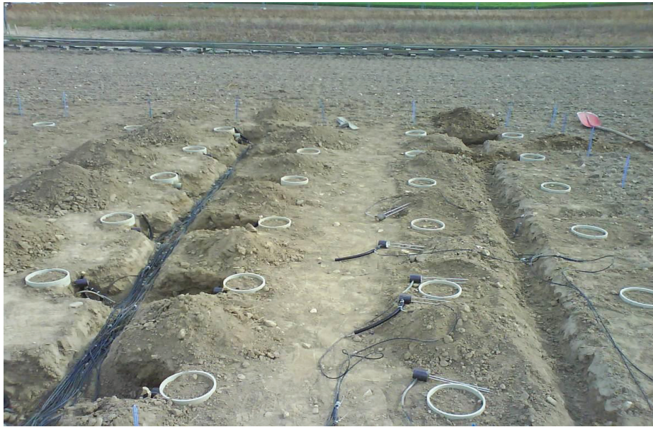
Figure 4.1: TDR probe installation for the field experiment from 15 th to 26 th of September 2008.
