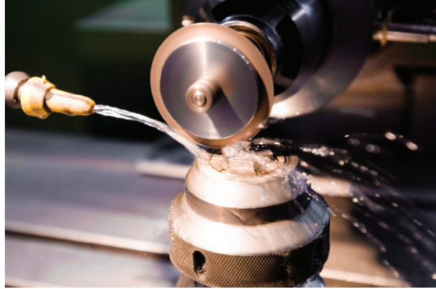
Figure 1.4. View of a working diamond cutting wheel with water coolant to remove chips [120].
