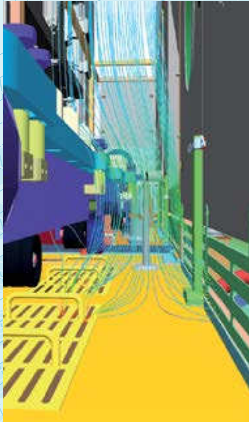
Figure 1: Laminar Airflow in the loading side of a lyophilizer.
