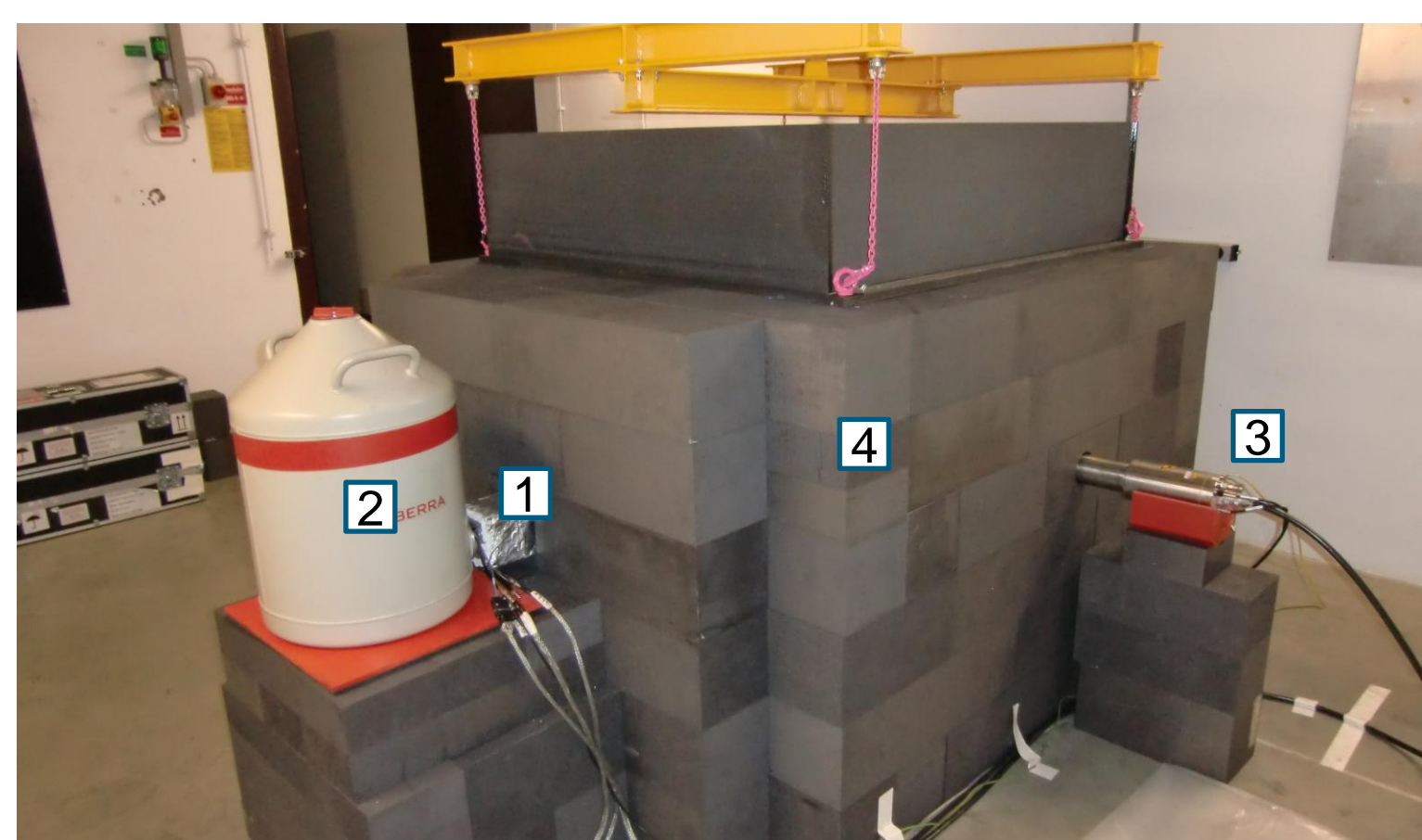
Fig. 4: The MEDINA test facility 1 HPGe detector with neutron shielding 2 Dewar with liquid nitrogen 3 Neutron generator 4 Graphite chamber
