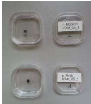
Figure 6.1: Samples of n-type semiconductor material \text{Mg}_2\text{Si}_{0.4}\text{Sn}_{0.6} and p-type semiconductor material \text{MnSi}_{1.85} .
