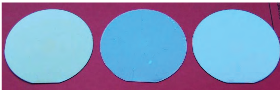
Figure 4.25 \text{ZrO}_2 , 3YSZ and 8YSZ thin layers deposited on silicon wafers
