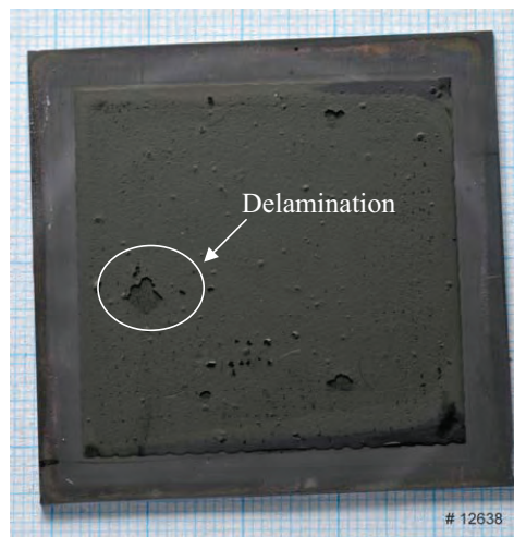
Figure 4.83 Pictures of an electrochemical tested single cell with 1 \mu\text{m} electrolyte and an LSC cathode
