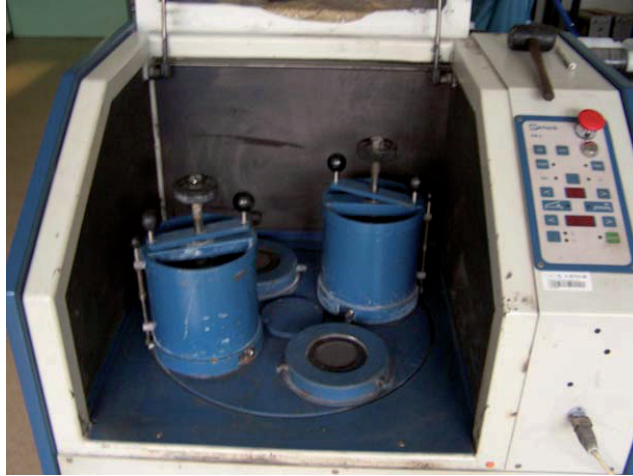
Figure 3.2 Schematic of planetary ball mill in the assemble situation in this work
