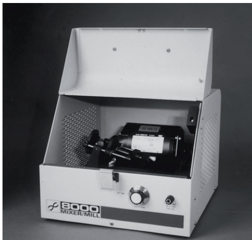
Figure 3.1 Schematic of SPEX 8000 mixer/mill in the assembled condition [64].
