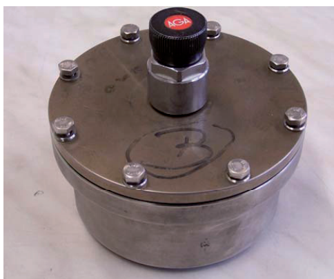
Figure 3.5 Photo of one of the hardened steel milling containers used in this work
