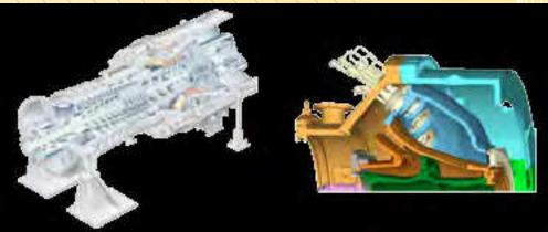
Figure 1: Gas turbine with can combustion system (lhs) vs. annular combustion system (rhs)
