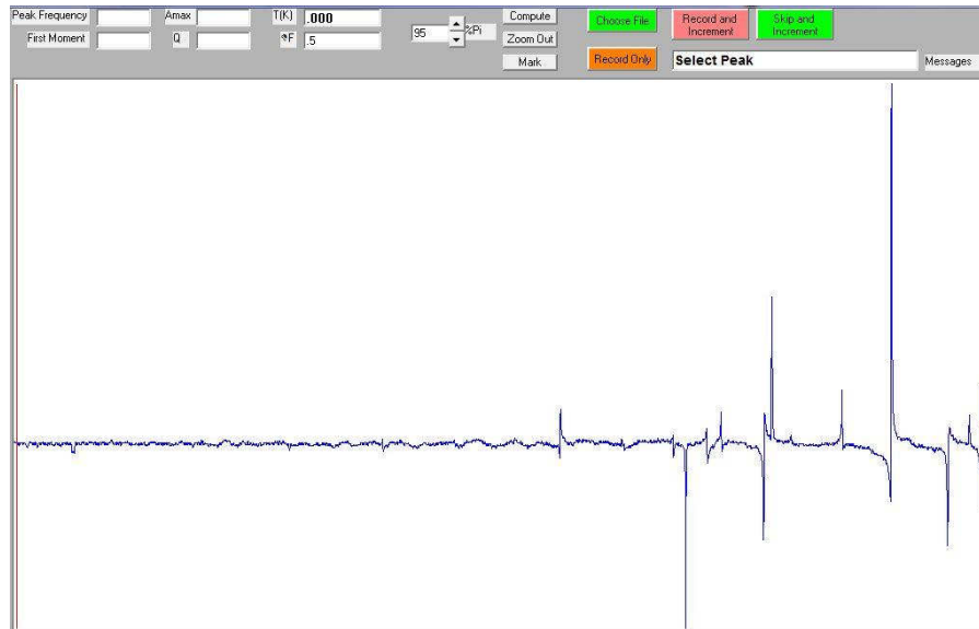
Image 35: RUS spectrum of "pristine" steel shown in RUS reduction program
