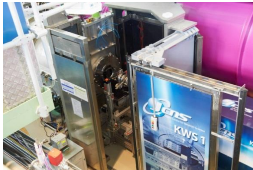
Image 24: Sample location in KWS-1 real set-up (photographed by Wenzel Schürmann/TUM)
