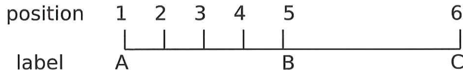
Figure 4.6 – Each number represents a position on the label. In other words, each number represents a distance between sputter gun and sample. The distance between A and B is equally divided by position 2, 3, 4.
