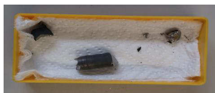
Figure 4.3: a) The cylindrical ingot of \text{MnFe}_4\text{Si}_3 . b) The broken ingot of \text{Mn}_4\text{FeSi}_3 .
