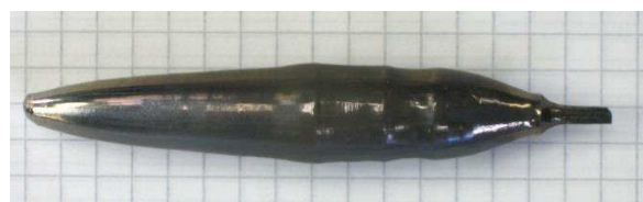
Figure 4.3: a) The cylindrical ingot of \text{MnFe}_4\text{Si}_3 . b) The broken ingot of \text{Mn}_4\text{FeSi}_3 .
