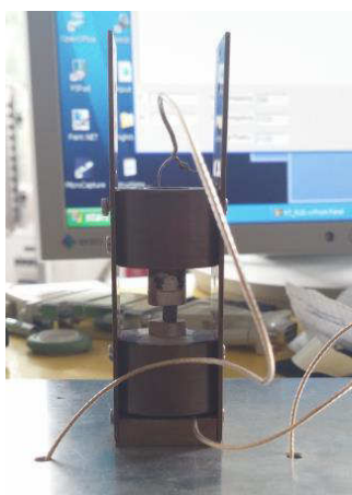
Figure 5.2: The setup for RUS measurements at room temperature.
