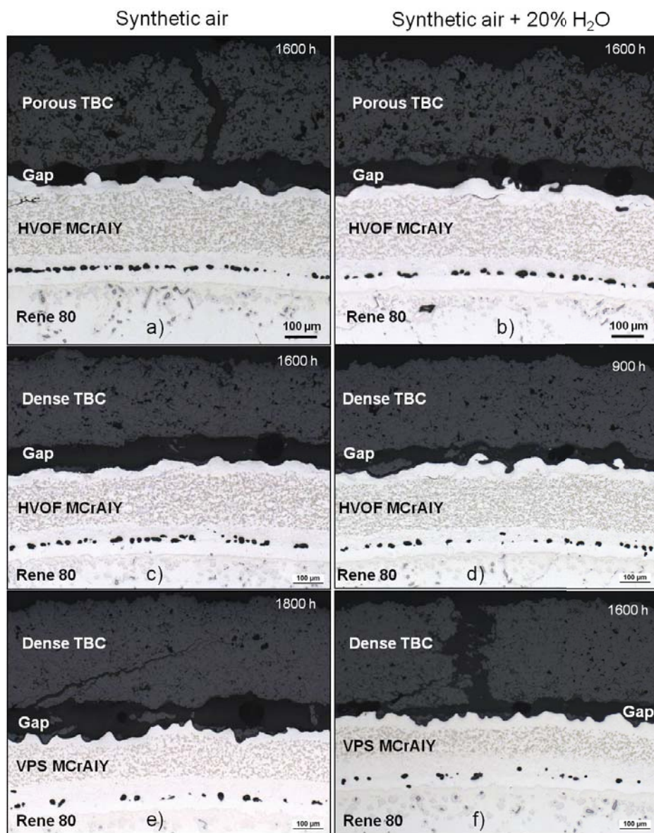
Figure 8.19 Metallographic cross sections of APS TBC systems with: HVOF bondcoat + porous TBC (a and b), HVOF bondcoat + dense TBC (c and d) and VPS bondcoat + dense TBC (e and f), after discontinuous exposure at 1050°C in: dry synthetic air a), c), e) and synthetic air + 20%H 2 O b), d), f) till TBC failure
