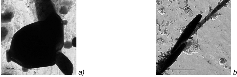
Figure 3 TEM micrograph of extraction replica: a) \text{Cr}_3\text{Ni}_2\text{Si}(\text{C},\text{N}) carbo-nitrides in DMV310N ( 586÷612°C): b) Laves ( \text{Fe}_2\text{W} ) in Sanicro25 ( 579÷605°C) .
