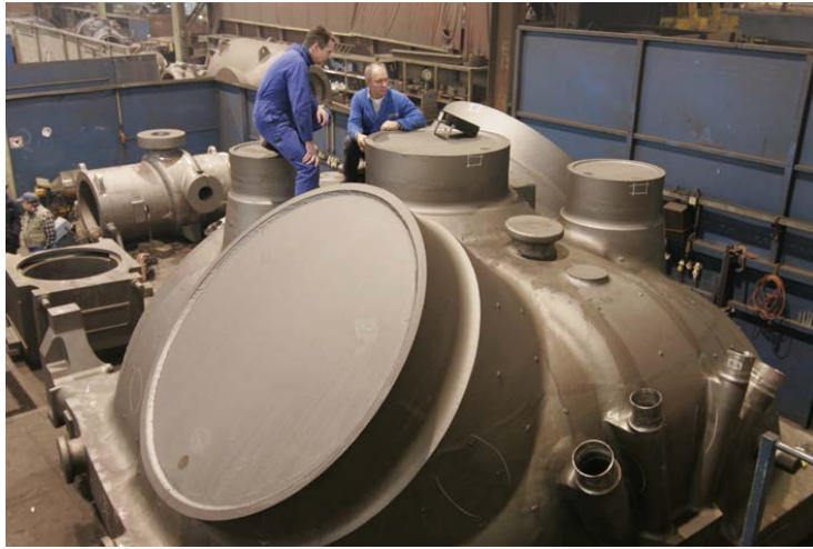
Figure 9 Outer casing top part during acceptance by customer and third party (non-destructive ultrasonic testing)
