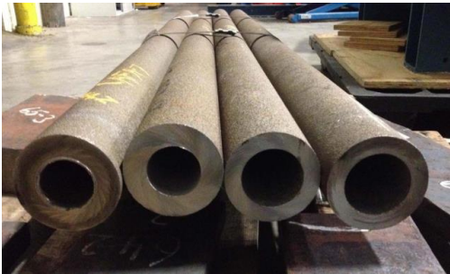
Figure 12: Centrifugal cast AFA tubes with 90mm OD x 16-19 mm WT x 1800 mm L (courtesy from Duraloy Technologies, Inc.).
