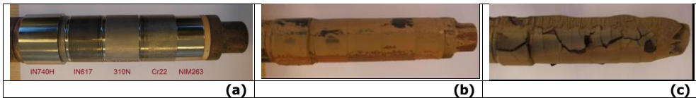
Figure 5: Fouling probe: a) samples before exposure; b) after campaign 1; c) after campaign 2.
