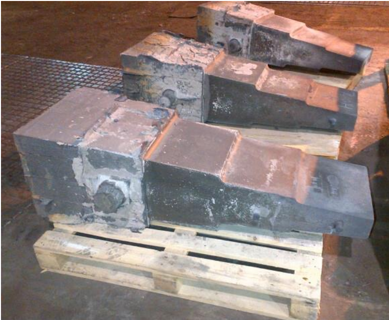
Figure 4 - Modified cast alloys after knock out of the mould
