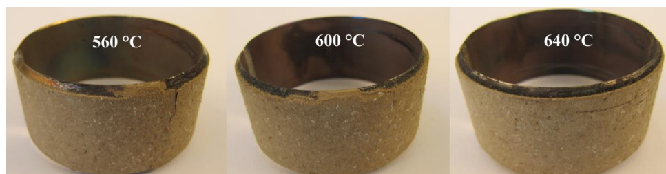
Figure 2. The windward side of the REF samples showing the deposit for all temperatures.
