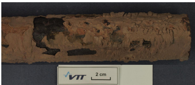
Figure 3: Overview of corrosion probe after testing campaign
