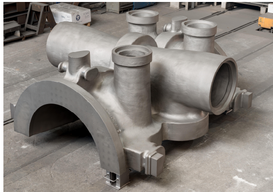
Figure 4: IP inner casing for advanced coal-fired steam turbines, material grade: CB2, made at voestalpine Foundry Linz in 2013
