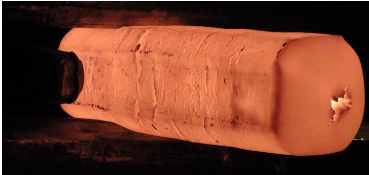
Figure 10: Mock-up of Alloy 282 Forging Manufacture
