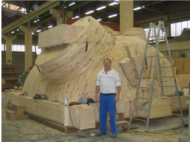
Figure 4 Wooden pattern for outer casing, upper half with steam outlet
