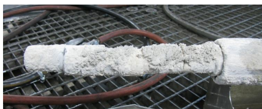
Figure 3: Metal rings covered with thick deposit layer after the 30 h exposure in the combustion chamber of the KSVa test rig.
