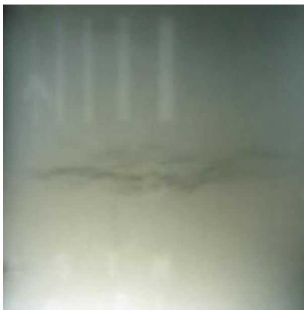
Figure 2 - Cracking detected by RT in a 180mm section thickness area of the cast alloy 282 step block. Similar defects were seen in the cast 740H step block. Cast alloy 263 passed RT examination but surface inspection showed deep surface crazing.
