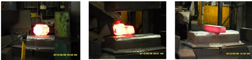
Figure 4: Forging of MarBN Trial Billets.
