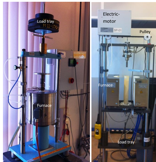
Figure 1. The two different types of SP creep test machines
