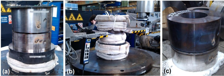
Figure 8: Welding of A263 + COST F Ø500 mm. Two counterpieces before welding (a), welding process (b), finished weld joint (c).
