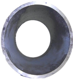
Figure 16: Interior view of a pipe after experimental rolling
