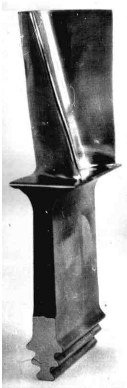
Fig. 1: The stationary turbine rotor blade (nickel alloy KhNi64WmoCoAlTiL, which is used for example instead of IN738 for hot part elements of gas turbine GTN 25 I at compressor stations (Pipeline Russia-EU))
