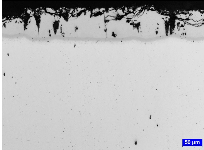
Fig. 2: Micrograph of a coating on FB2, sand blasted substrate
