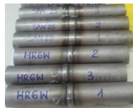
Figure 1: The welded tubes as delivered from RAFAKO S.A: Sanicro 25 OD 38 x 8,8 by SANDVIK, HR6W OD 38 x 8,8 by SMI.
