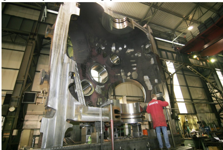
Figure 7 Outer casing half during rough machining
