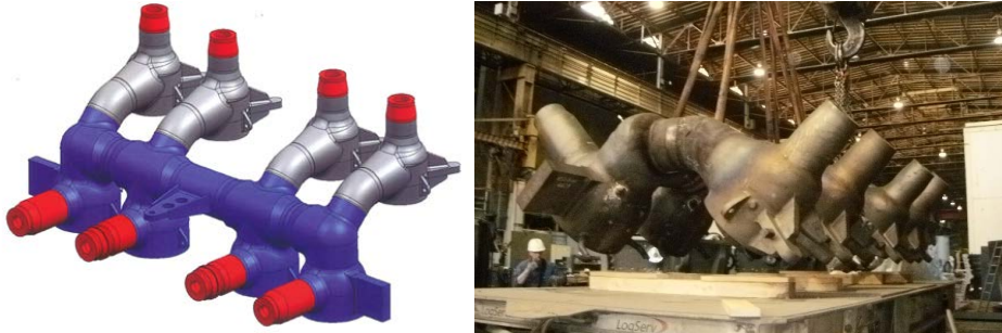
Figure 16 9 cast- and 8 forged components welded together for a main steam valve
