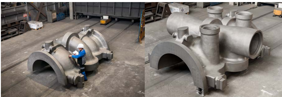
Figure 17 Biggest CB2 casings: IP-inner casing upper half (34tons) and lower half (34 tons)
