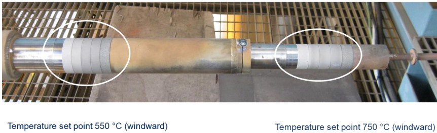
Figure 2 : VTT's high temperature probe for two measurement temperatures.
