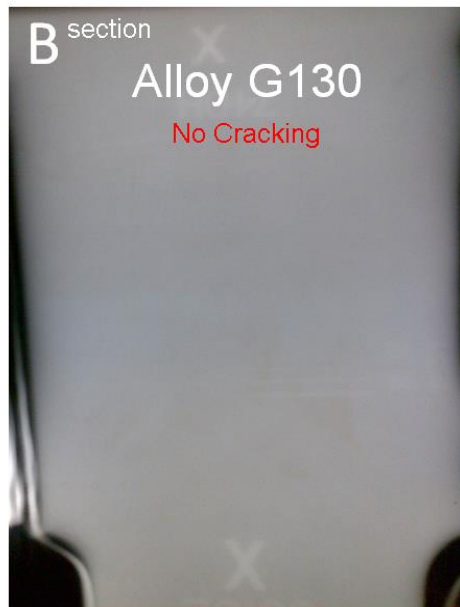
Figure 5 – RT graph of G130 step block
