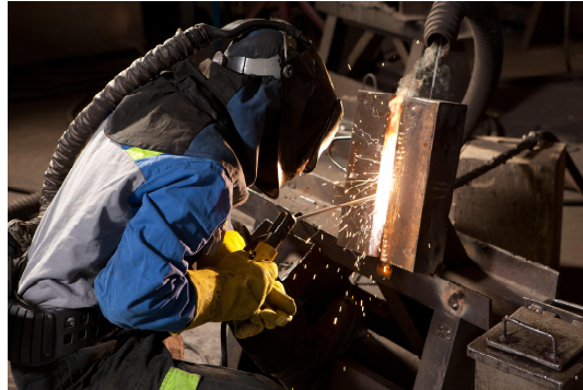
Figure 3: SMAW with CB2 filler for Welding Qualification at voestalpine Foundry Linz
