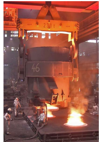
Figure 5 Casting with a heavy ladle (150 tons of molten metal), fully alloyed in the LD steelmaking plant
