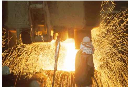
Figure 3 Casting at voestalpine Giesserei Linz GmbH, with a 50 ton ladle
