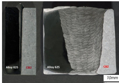
Figure 5: Dissimilar welding of A625 cast and CB2, comparison between electron beam and stick welded joints, wall thickness 50 mm, voestalpine Foundry Traisen, 2013
