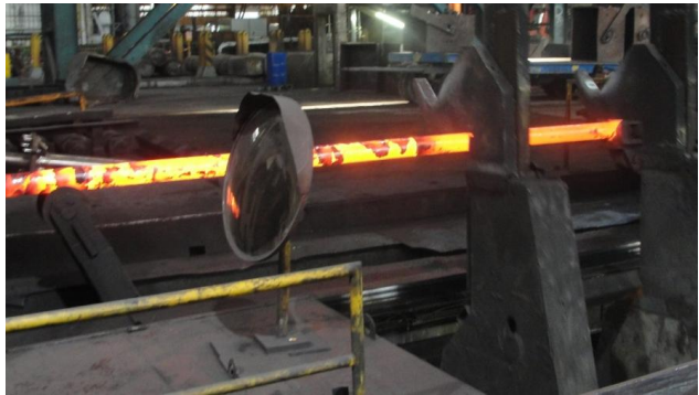
Figure 6: Bar production of modified austenitic stainless steel [CAS]
