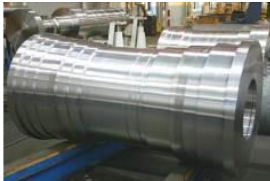
Figure 9: Quality heat-treated and machined FB2 Forging; delivery weight 9.2 tons
