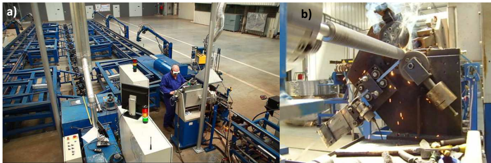
Fig. 8. Laser welding station [24] (a), Laser welding of finned tubes (b)
