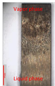
Figure 10: Sample partially immersed in the salt
