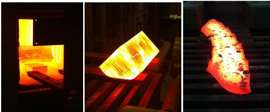
Figure 3: MARBN pilot full-scale pilot ingot obtained at Cogne steelwork (left) and preliminary cutting plan (right).
