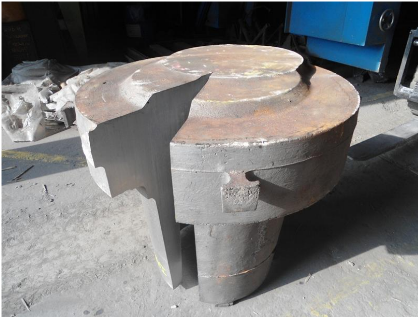
Figure 6: MarBN cast bonnet manufactured by Goodwin Steel Castings Ltd within the UK IMPACT project. The reason of a sectioning a 30° cross sectional slice out from the bonnet was to conduct mechanical testing.
