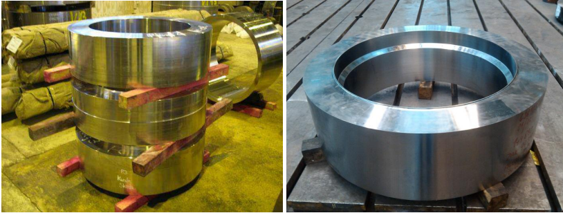
Figure 10: Rings for demonstration of rotor welding taken from full-scale rotor from A263 with diameter of 1000 mm.
