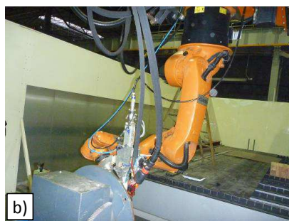
Fig. 3. Station for technological tests of laser and hybrid welding of the DMV 617 mod alloy, Energoinstal SA
