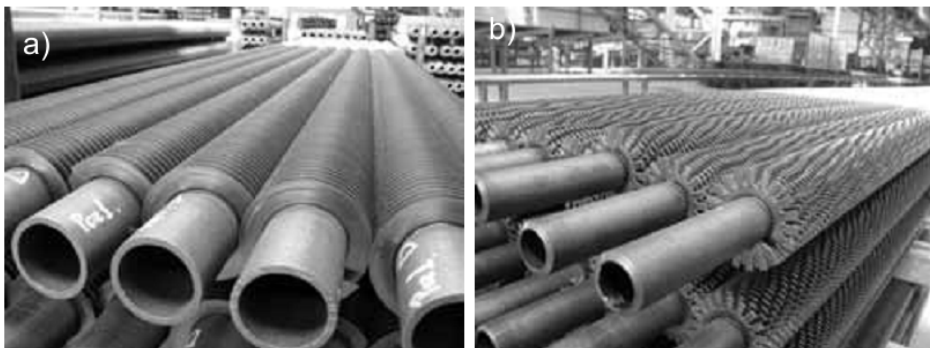
Fig. 1. Welded finned tubes with solid (a)[5] and serrated (b) fin [5]
