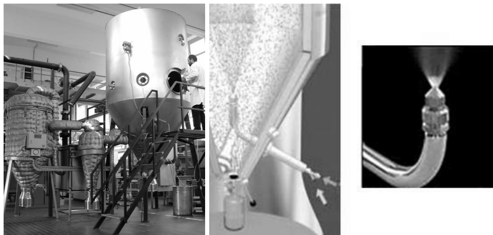
Fig. 2: Niro 6.3-SD Spray dry plant and 2-fluid nozzle configuration at VITO
