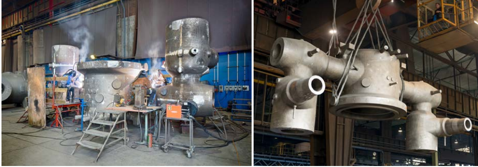
Figure 15 High-pressure outer casing with welded-on valves ( 31\text{ t} + 2 \times 19\text{ t} = 69\text{ t} )
