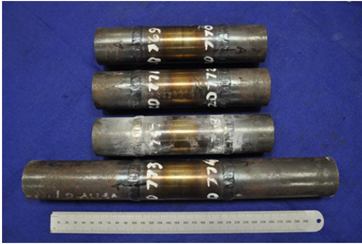
Figure 5: MarBN Tubes samples ready for insertion in power plant for long term testing.
