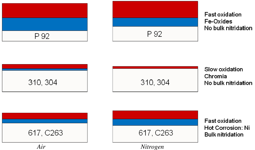
Figure 15: Summary of scale formation of alloys investigated in this work, air (left) nitrogen (right)
