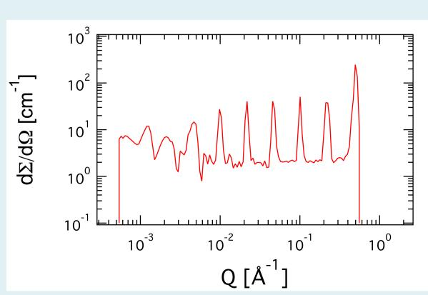
Plot of  $\delta$ -peaks over SKADI's complete Q range. FOM gains compared to D22 are 36. This gain includes the improved Q resolution.
