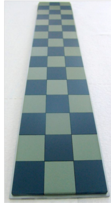
Fig. 16. ITO/AZO mosaic target (chess pattern) for sputtering tests under industrial conditions at VHF Technologies. Dimension 750 \times 125 \text{ mm} , 48 segments.
