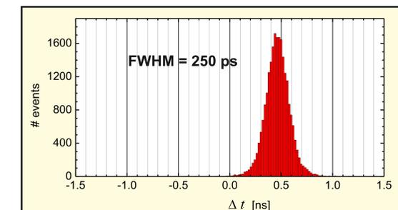
The Coincidence Peak obtained from 2 Dies shows a FWHM of 250 ps. With careful skew correction this can be achieved for the complete scanner.
