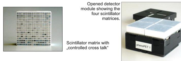
Opened detector module showing the four scintillator matrices.
