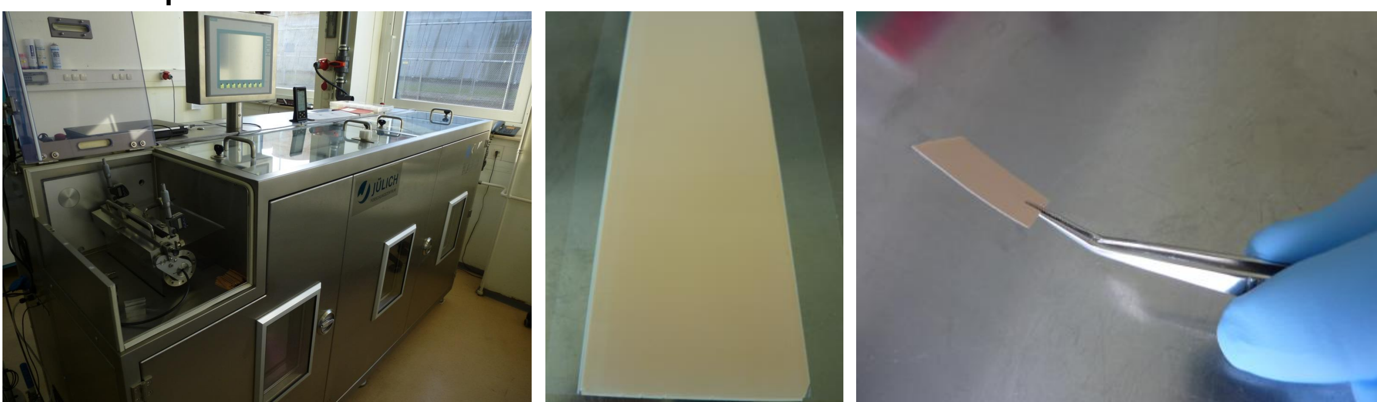
Fig.2: A tape casting line at IEK-1 (l.) can be used for large scale tape casting. Al-LLZ tapes were successfully processed by tape casting with a gap size of 250 \mu\text{m} (m.) and 500 \mu\text{m} . Solid electrolytes with a green tape thickness of 90 \mu\text{m} (r.) and 180 \mu\text{m} were used for further sintering studies.
