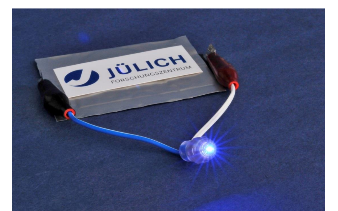
Fig.6: Bulk prototype all-solid-state lithium battery.
