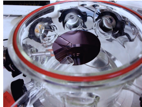
Figure 17: Wafer-scale deposition of self-assembling organic monolayers possible in GLOBUS device.
