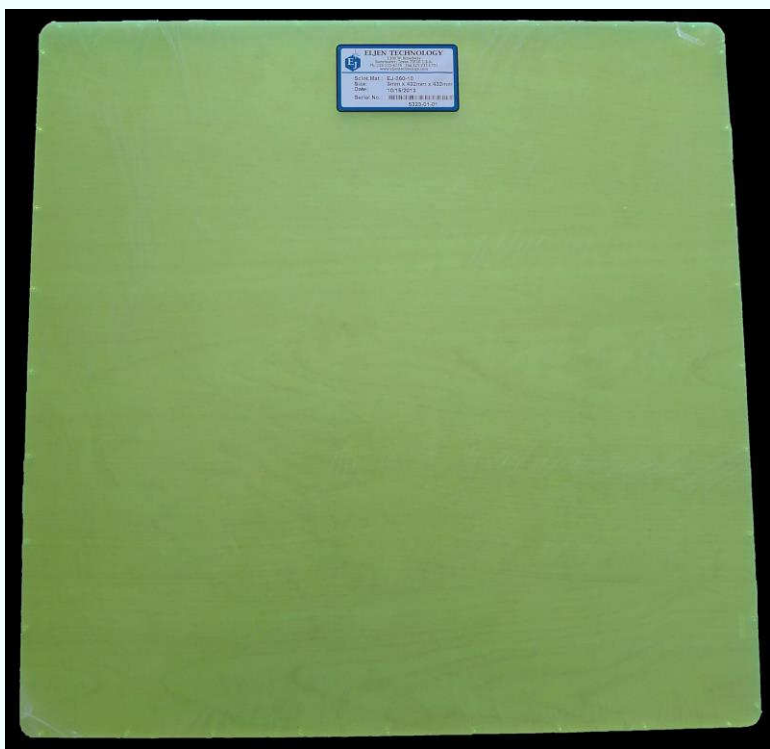
Fig. 2: General purpose plastic scintillator used for fast neutron detection via recoil protons.
