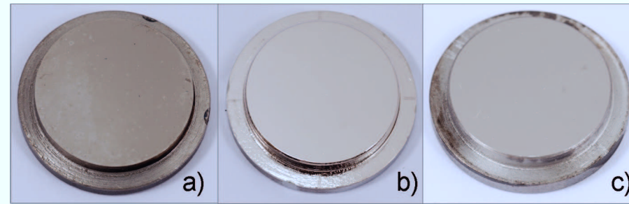
Figure 5.1. Photographic view of mirrors from set 1 before exposure: a) Mo coating on polycrystalline Mo substrate made by evaporation technique, b) Rh coating on polycrystalline Mo substrate made by evaporation technique, c) SC Mo mirror.
