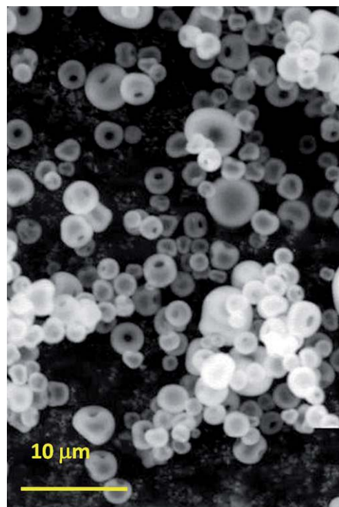
Fig. 2 Scanning electron micrographs of self-assembled grains of only silica colloid. It is evident that the grains are either just about to be smooth doughnuts or nearly spherical but no deformed doughnut is observed as is observed for the silica– E. coli system.
