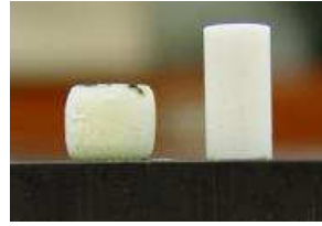
Fig. 15 Sample tested at 800 °C with 43 % strain in comparison with a non-tested sample [Liu 2011]
