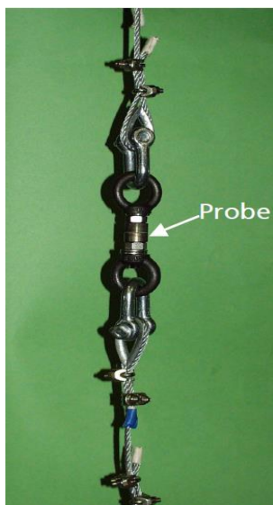
Fig. 16 Joined samples in the tensile strength measurement set-up [Sch 2002b]
