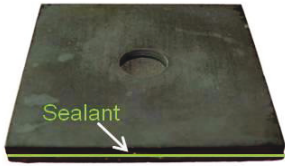
Fig. 20 a) Sandwich sample formed of two Crofer22APU plates of 50 x 50 mm 2 dimension joined by glass-ceramic sealant. b) Schematic view of a sandwich sample open with the applied sealant
