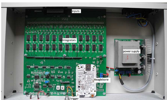
Fig. 1: Inside of the multichannel pico amperemeter module. The white PCB is the BEAGLEBONE providing TCP/IP connectivity.
