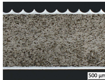
Figure 8.1: Polished cross section of a specimen used for bending testing. Experiments were performed on riblet structured 1.6 mm thick Alclad 2024 sheets with a riblet diameter of 300 \mu\text{m} . The specimens were of the same type like in Fig. 5.2d (p. 45).
