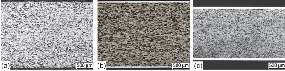
Figure 4.4: Polished cross sections of studied AA 2024 specimens. (a) 2 mm thick bare sheet. (b) 2 mm thick clad sheet. (c) 1.6 mm thick clad sheet.
