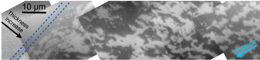
Figure 5.13 – Survey XMCD image of a 60 ML \text{Ni}_{38}\text{Pd}_{62} wedge. The image shows film thicknesses from \sim 5 ML - 60 ML. Magnetic contrast in domains is in-plane, while on the left-hand image side the non-magnetic phase can be seen. An in-plane monodomain can be seen at the onset of the magnetic contrast.
