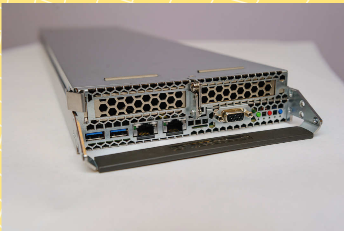
Figure 2: A V210S compute node as used in the JURECA cluster. Each node hosts two CPU sockets. The V201F version, which has twice the width of a V201S module, can additionally host two PCIe-based accelerator cards.
