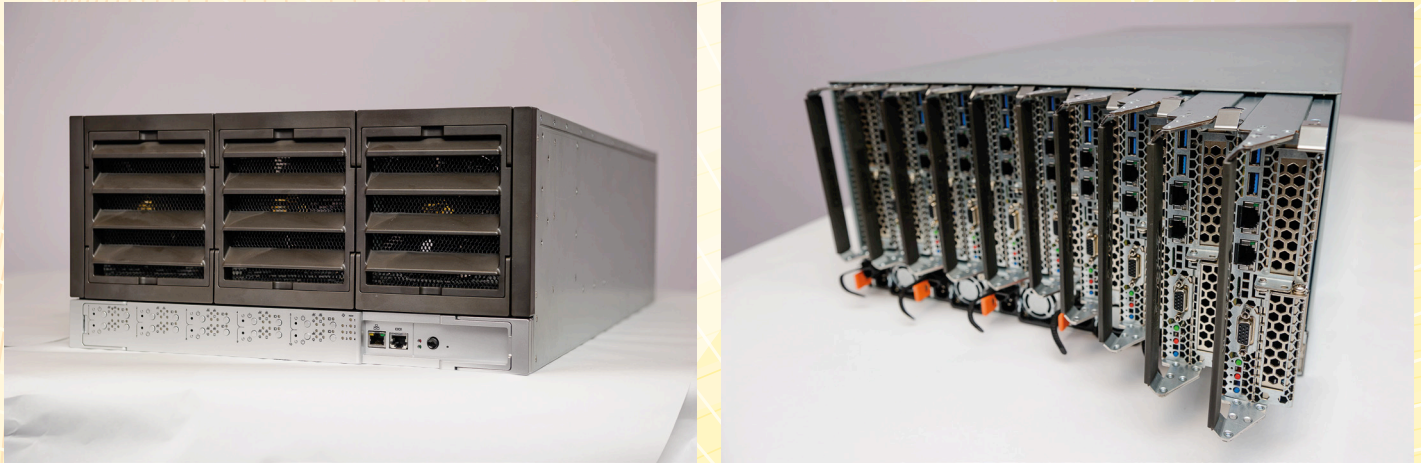
Figure 1: (Left) Front view of a V-class enclosure. (Right) Rear view of a V-class enclosure hosting ten V210S compute nodes (slim or fat nodes of type 1 in JURECA). The same chassis can host five V210F accelerated compute nodes occupying twice the space of V210S node.
