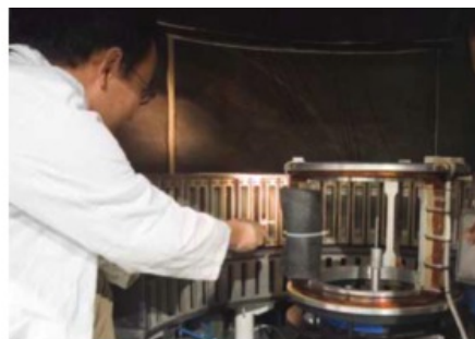
Fig. 6: (left) Magnetic field setting in a xyz-coil system for an adiabatic nutation of the polarization of cold neutrons in horizontal x-direction at the sample turning to a vertical (guide) field B_z at further distance from the sample. (right) A photo of the xyz-coil system in the DNS instrument at the FRM-2.
