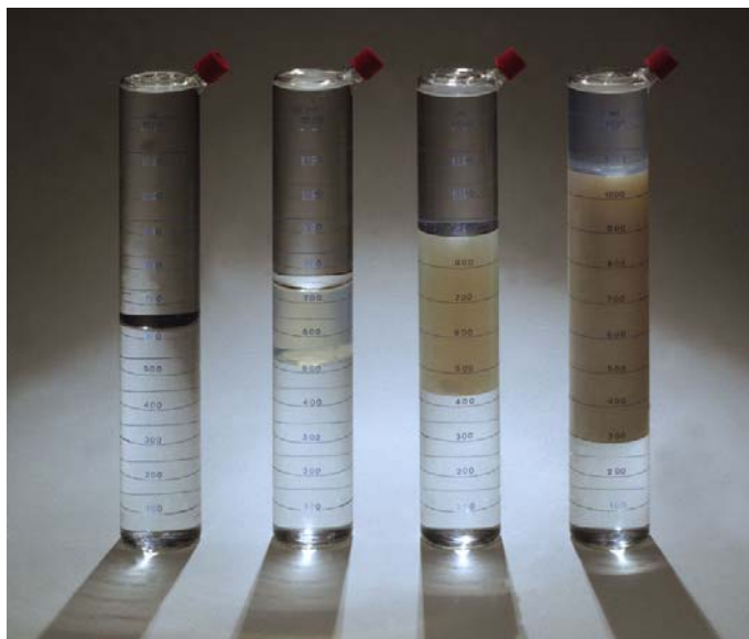
Fig. 19: Effect of small amounts of amphiphilic block copolymer PEP-PEO (compare Fig. 21 below) on the phase behavior of balanced microemulsions. Far left: oil-water coexistence. Left: 7 weight % surfactant C_{10}E_4 produce a three-phase coexistence with a microemulsion phase in the center. Right: 0.5 weight % of PEP5-PEO5 increase the microemulsion volume two-fold. Far right: 1.0 weight % of PEP5-PEO5 increases the microemulsion volume three-fold (preparation and photo: J. Allgaier).
