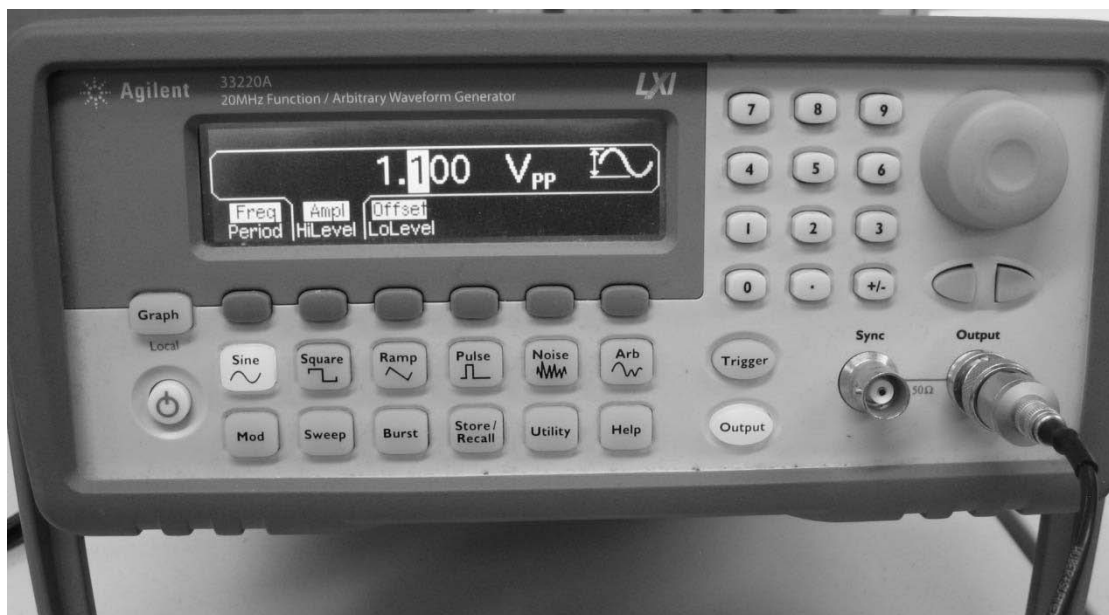
Figure 9.3 A function generator is sued to generate a sinusoidal signal. The signal with amplitude of 1.1 V was sent to the aiNCAP using sound card upon receiving the send command from JNCAP to aiNCAP
