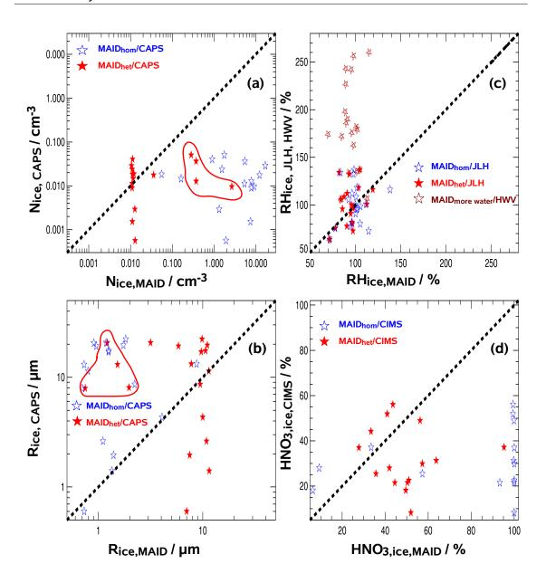
Figure 4.8: Overall closure – comparison of MAID results with in-situ observations (stars: MAID results for 'best' – red, 'homogeneous' – blue, and 'more water' – burgundy vs. observations for a: ice crystal number density; b: ice crystal size; c: relative humidity with respect to ice; d: nitric acid in ice; encircled red stars represent the four trajectories that contain a subsequent homogeneous freezing event, see text).
