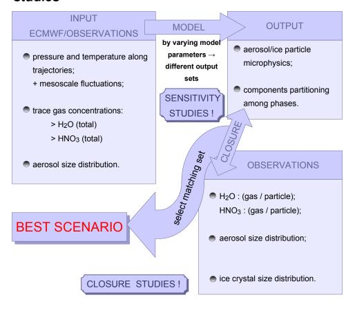
Figure 3.4: Operation scheme of MAID for sensitivity and closure studies.
