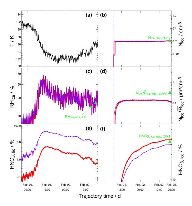
Figure C.5: Evolution of the CR-AVE cirrus along the selected trajectory in the 'bigger aerosol' scenario compared to the 'best' scenario (red: 'best', violet: 'bigger aerosol' scenario; a: temperature; b: ice crystal number density; c: relative humidity with respect to ice; d: number density · size of ice crystals; e: nitric acid in liquid aerosol; f: nitric acid in ice; dashed lines: appearance of first ice crystals; green triangles: observations).
