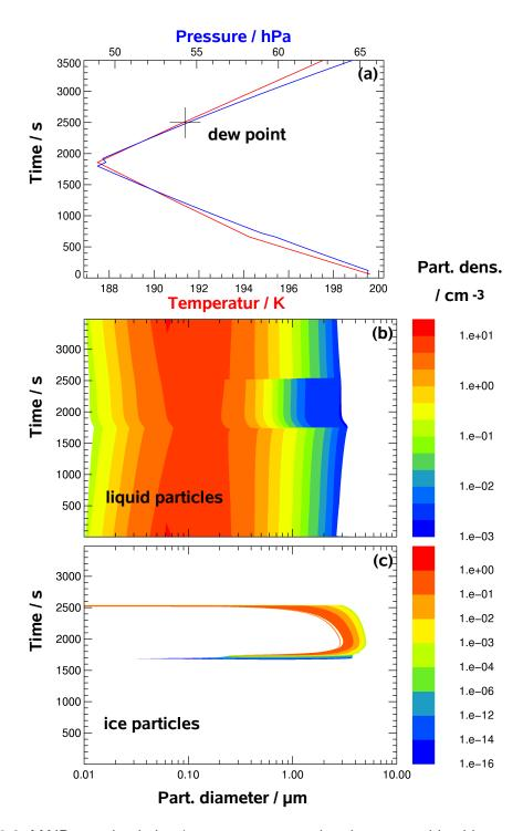
Figure 3.3: MAID test simulation (a: temperature—red and pressure—blue history of the air parcel; b, c: Lagrangian time evolution of the size distribution for liquid and ice particles, respectively; for details see text).
