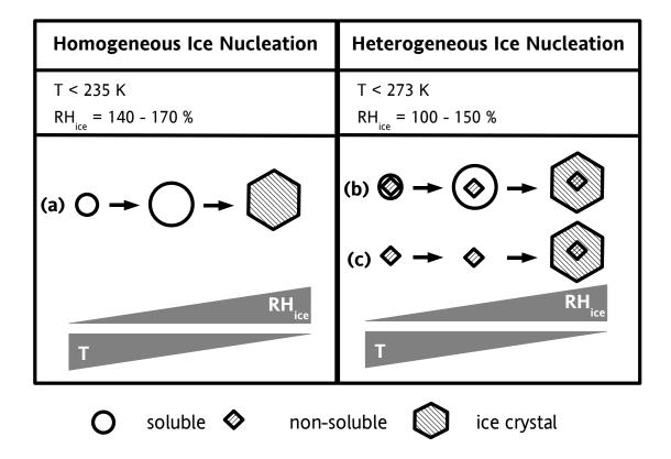
Figure 2.4: Pathways to ice nucleation in UT (a: homogeneous; b/c: heterogeneous immersion/deposition freezing, respectively)
