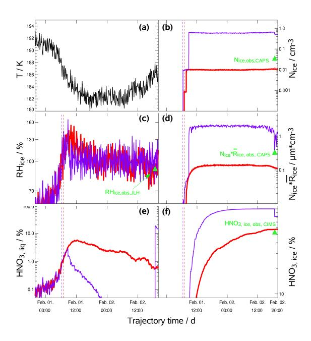
Figure C.3: Evolution of the CR-AVE cirrus along the selected trajectory in the 'higher temperature fluctuations' scenario compared to the 'best' scenario (red: 'best', violet: 'higher temperature fluctuations' scenario; a: temperature; b: ice crystal number density; c: relative humidity with respect to ice; d: number density · size of ice crystals; e: nitric acid in liquid aerosol; f: nitric acid in ice; dashed lines: appearance of first ice crystals; green triangles: observations).
