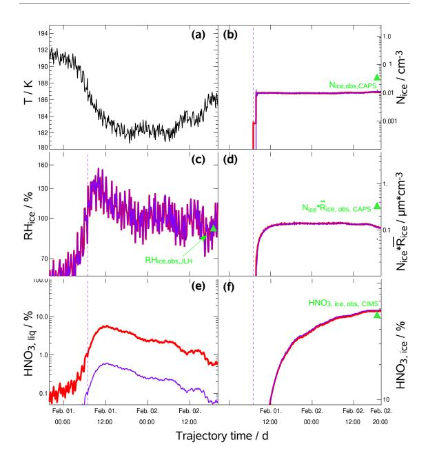
Figure C.6: Evolution of the CR-AVE cirrus along the selected trajectory in the 'few aerosol' scenario compared to the 'best' scenario (red: 'best', violet: 'few aerosol' scenario; a: temperature; b: ice crystal number density; c: relative humidity with respect to ice; d: number density size of ice crystals; e: nitric acid in liquid aerosol; f: nitric acid in ice; dashed lines: appearance of first ice crystals; green triangles: observations).
