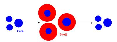
Figure 3.2: Preservation of aerosol material upon growth and evaporation in a 'full-moving structure'
