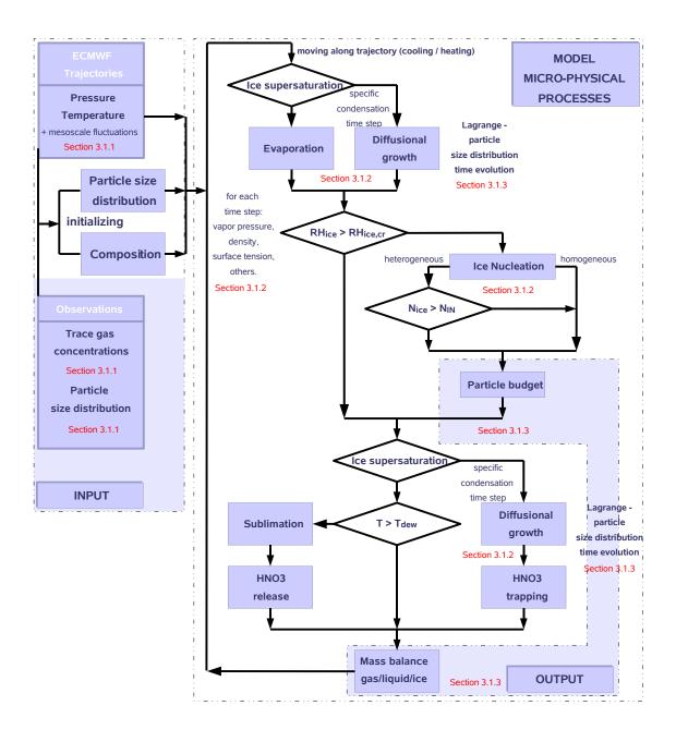
Figure 3.1: Flow chart of MAID (description of each element of the chart is given in the corresponding section, marked in reddish).
