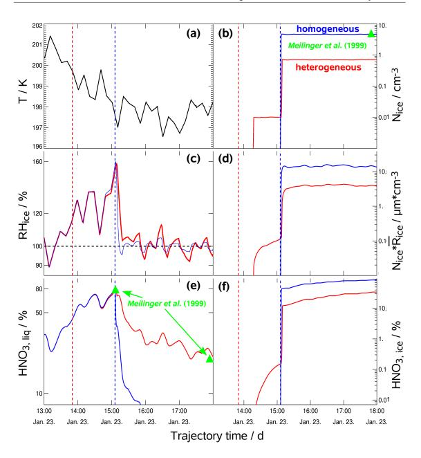
Figure 3.5: Evolution of an Arctic cirrus along an atmospheric trajectory, formed red: heterogeneously / blue: homogeneously (a: temperature – black; b: ice crystal number density; c: relative humidity with respect to ice; d: integral size of ice crystals; e: nitric acid in liquid aerosol; f: nitric acid in ice; dashed lines: appearance of first ice crystals; triangles: values presented by *Meilinger et al.* (1999), used in the MAID validation study).
