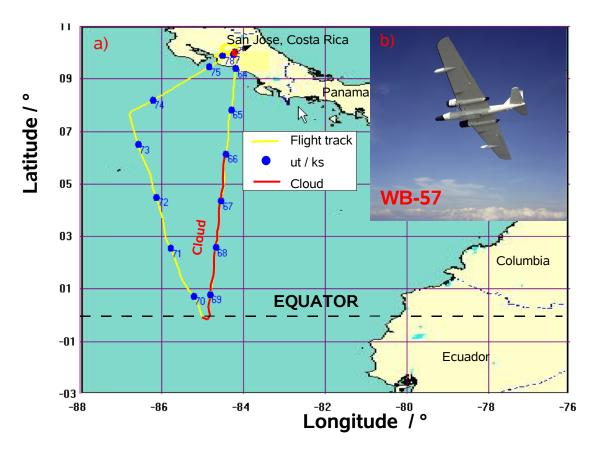
Figure 4.1: a: CR – AVE flight track on 2<sup>nd</sup> February 2006 (yellow line: flight track; red line: cirrus cloud; blue dots: universal time in ksec); b: NASA WB – 57 high altitude research aircraft.
