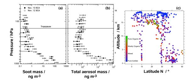
Figure 5.1: Vertical profiles of soot and total aerosol mass concentration, fraction of organics in the total aerosol (a: vertical profile of the soot mass concentration; b: vertical profile of the total aerosol mass (*Schwarz et al.* (2006)); c: an altitude - latitude cross-section of the organic fraction in the total aerosol (*Murphy et al.* (2006))).
