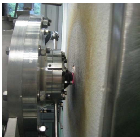
Figure 11. Flow channel furnace coupled with the MBMS.
