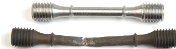
Fig. 6.71: Images of the specimens of KCP before and after testing at 700°C and 10MPa.
