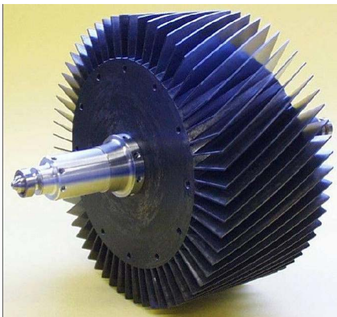
Fig. 14.6: Photo of the velocity selector drum of the JCNS instrument KWS-3 showing the screw-like twisted channels separated by absorbing walls, which only neutrons of a certain wavelength band can pass when the drum is turning.
