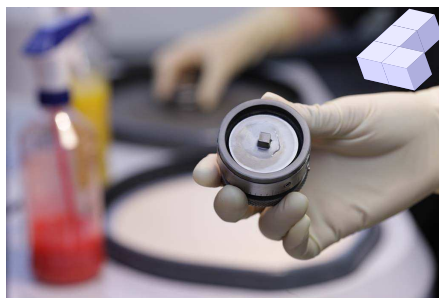
Figure 34: A snapshot during polishing of a bulk polycrystalline sample mounted on the polishing holder. Inset: a figure of the 'L' shape which is mounted on the sample holder to produce the third perpendicular face, see text. Courtesy: Forschungszentrum Jülich.
