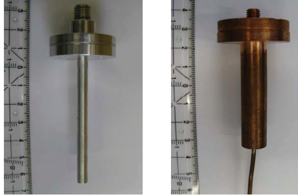
Figure C-1-3 Typical Al (left, diameter: 4 mm) and Cu (right, diameter: 9 mm) sample holders used for powder sample measurements on DNS.
