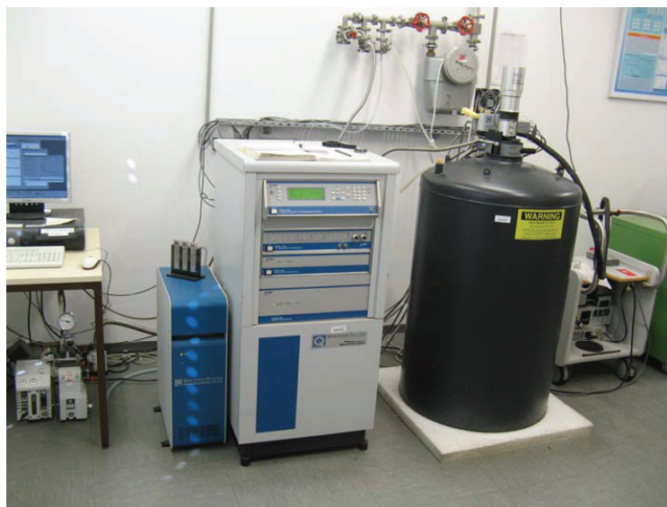
Figure C-6-1 Picture of Quantum Design PPMS, which is running heat capacity measurement equipped with a dilution insert.
