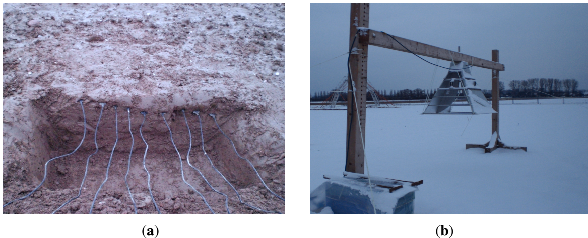
Figure 2. Decagon EC-TM capacitance probes were installed near the footprint of the ground-penetrating radar (GPR) antenna in a trench to monitor the vertical and lateral dynamics of soil temperature and dielectric permittivity (a), and the fully-automated off-ground GPR setup with an antenna fixed at 110 cm above the ground (b) (after [42]).
